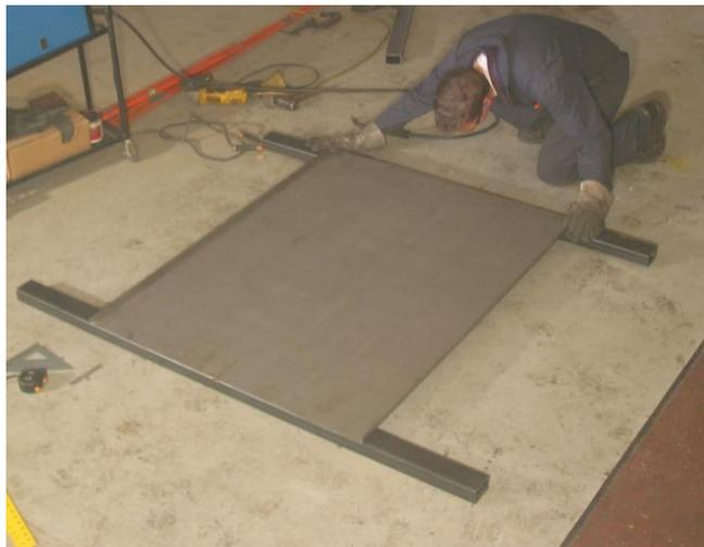
Mark a center mark on the rear bed tube (longest) on the top of the back side. Also mark the center of the front of bed tube. Locate the bed sheet metal piece and mark the center on the front and back (bends are on the left and right sides for your reference).
