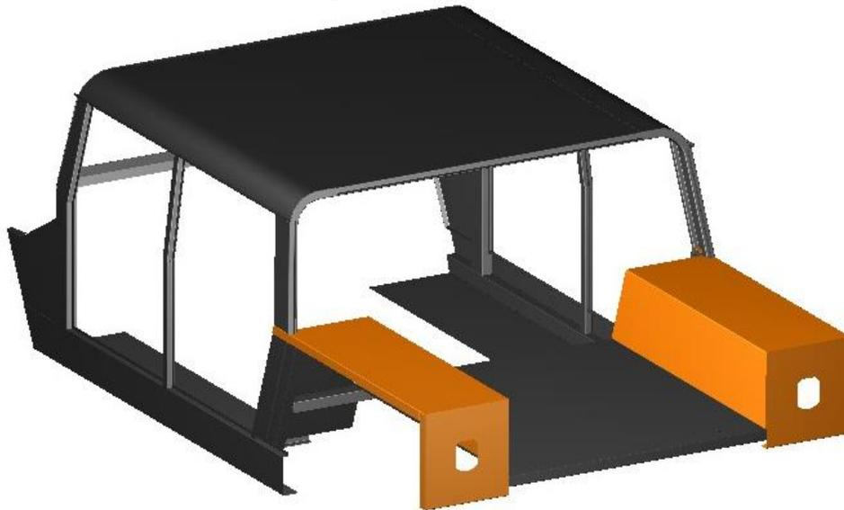
Next find the right taillight plate (curved side goes downward and bent edge goes on outward side). Tack the taillight plate to the right bed side piece. Using the outer edges and inside corner as a guide.
