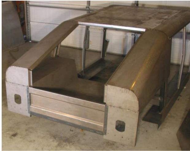
Position the tailgate side and bottom supports into place and grind for precise fitment. It is a good idea to work on a flat surface and align the flat sides down. You may even want to clamp down the tailgate to flatten the sides and then tack the side, bottom, and other side supports which can then hold the tailgate in a flat position. Once you have all the parts in place and everything is correct then you can then finish weld.
