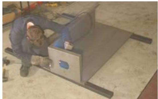
Another trick is to tack and then hammer the metal into place while the tack is hot. This can be useful when pulling a part into location. This only works if you gently hammer immediately after the weld. If the weld cools then you will probably need to cut off the tack and start over as it can leave an island of weld that will keep the part from going into place and may damage body skin if you hammer hard or once cooled.
