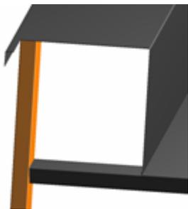
You may want to have the tube about an 1/8th of an inch under the edge of the sheet metal to leave room for the back seat pedestal that will fit into that area later. You can tack the top of the tube into place so you can align the middle part to the front of the bed front cross tube and tack into place.
