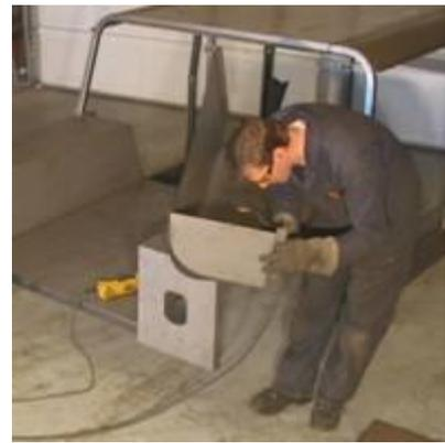
Once you have both SlantBack sides ready to place on the body then you can start to position into place. You will want to measure the width of the bed area so you can mark the top for where you will be fitting the side pieces.
